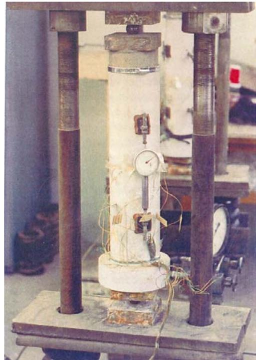
Fig. 4. Testing of freshly-placed concrete in a plastic form under the prolonged action of pressing
