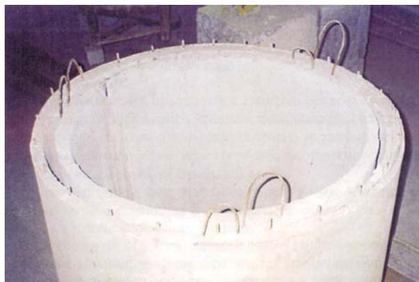
Fig. 7. Reinforced concrete cylindric shells of compound frame wall
