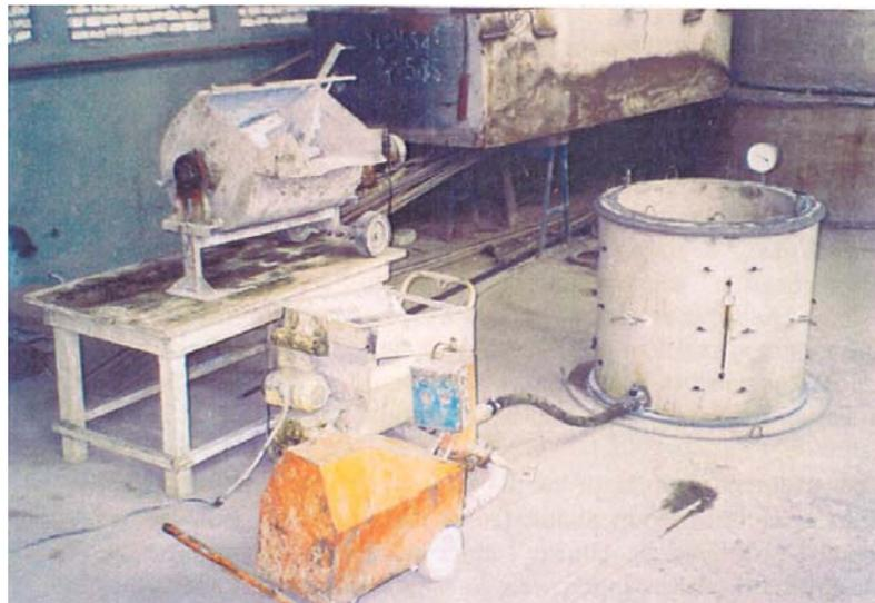
Fig. 8. Injection of cement grout into the gap of compound frame wall
