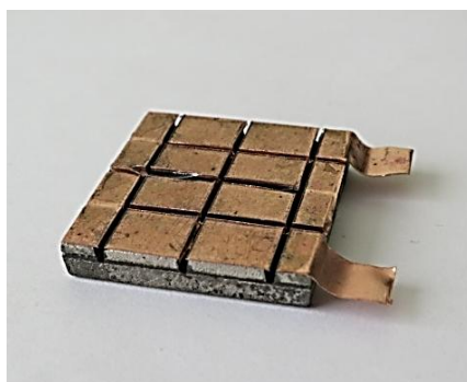
Fig. 5. Electric insulation node of a battery (1.3 x 1)
