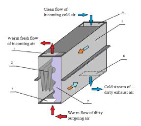
The design is a rectangle in the form of an elongated parallelepiped. Pipe (1), which is divided by a broken plane (2) into two upper and lower sections, each section has 2 slots, for the lower section there is a slot (5) and a slot (6), for the upper section, a slot (3) and a slot (4). The ribs of the fracture plane are parallel to the ribs of the pipe. The ends of the broken plane and the pipe are closed by a plane perpendicular to them (7).
