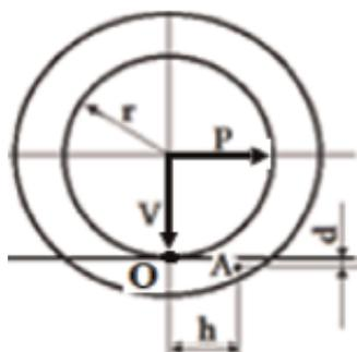
Fig. 9. Forces acting on the wheel axle
