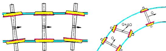
Fig. 1. Movement of the wheel-set in the straight and curve
