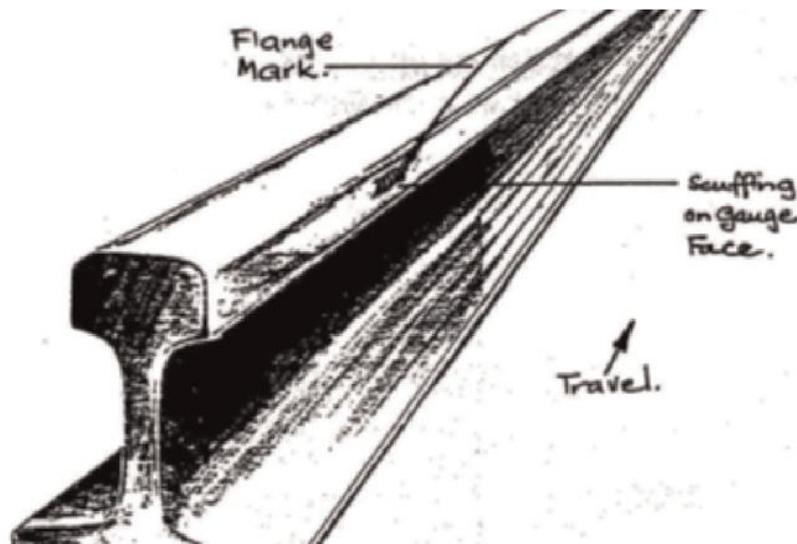
Fig. 3. The trace of the wheel climbing on the rail
