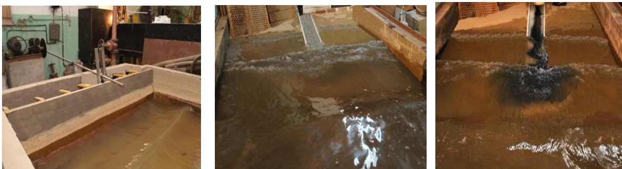
Fig. 5. Photos of laboratory studies of wave effects on pollutants brought into the sea by the river inflow
